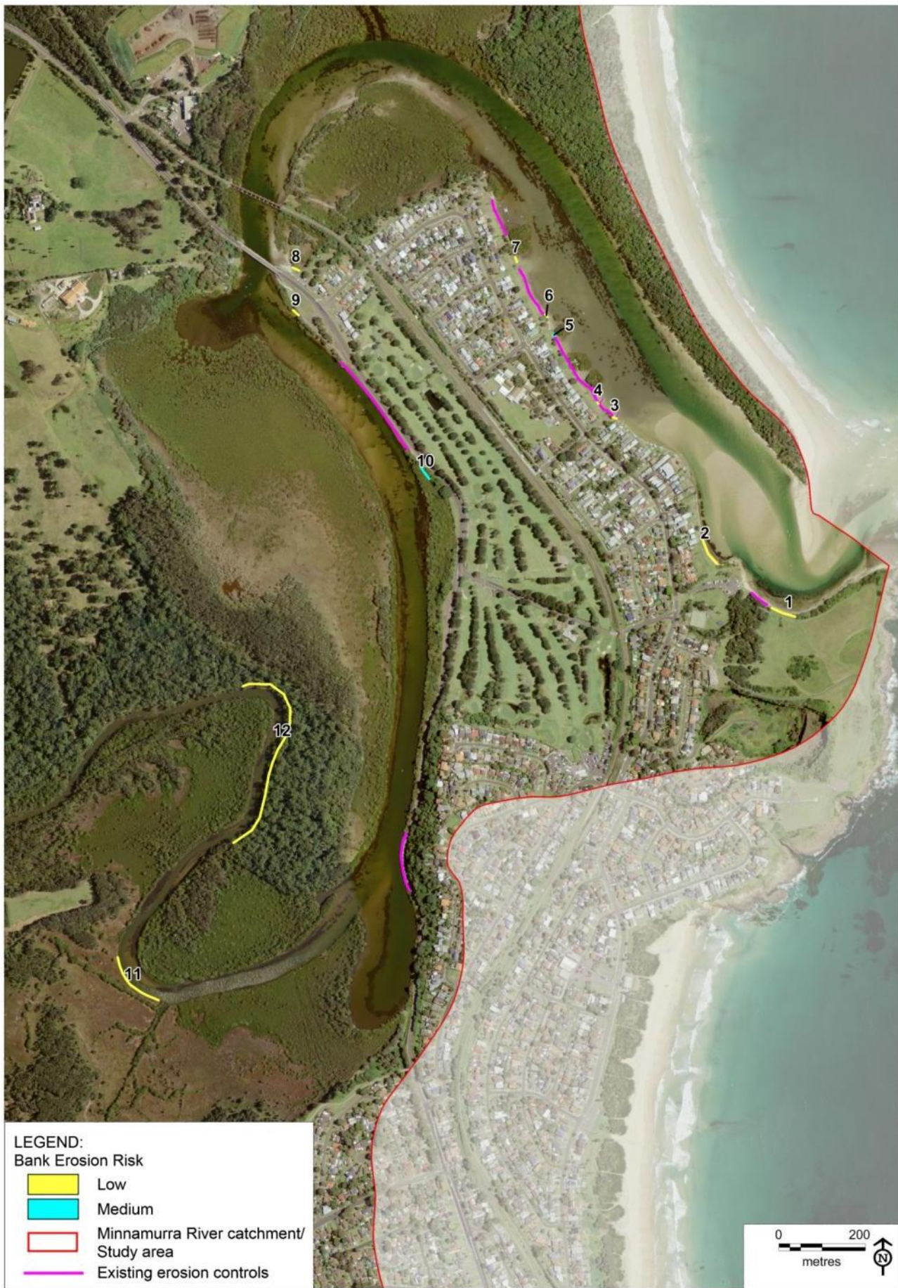
Figure 67: Locations of bank erosion sites in the lower to mid-estuary
