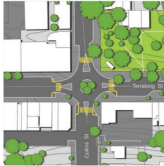
Figure 9.3: TCS Proposal for Bong Bong Street/Shoalhaven Street Intersection
